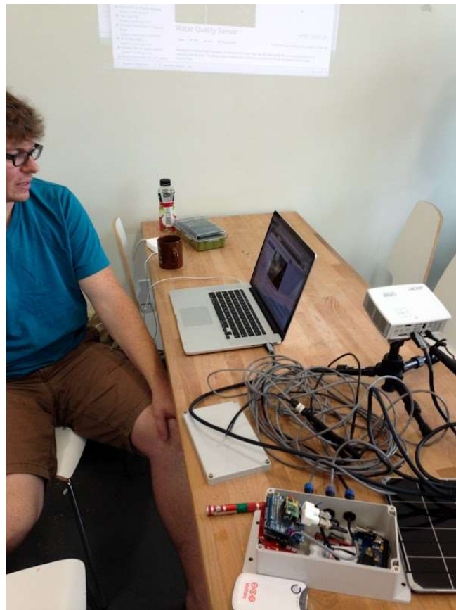
Leif Percifeld led a group discussion on water quality and showcased his latest low-budget DIY water sensing kit which used Arduino combined with probes measuring temperature, dissolved oxygen and conductivity. The kit transmits its data continuously over the cell network to the site xively . He developed the kit to measure sewage outfalls after storms in New York City. Jack Summers, a chemist in North Carolina, skyped in for part of this session to discuss progress on making a DIY potentiostat to test for heavy metals in water.
