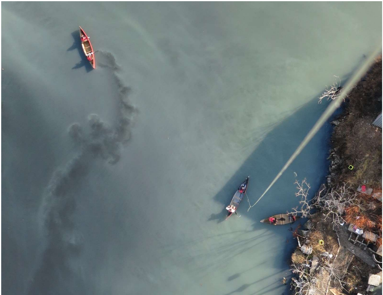
From a Public Lab research note by Eymund Diegal about mapping sewage flows in the Gowanus Canal. Note the people on boats doing the mapping and the balloon tether that links the camera and image back to their bodies.
